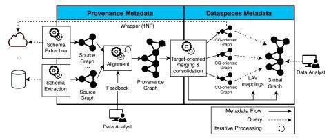
Fig. 1: High-level overview of the functionalities offered by Odin
